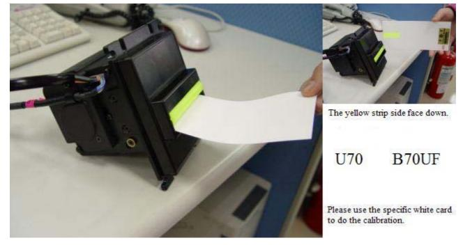
Input the B77UF/U77 white card for U77 and B77UF. Input the B85UF/U85 white card for U85 and B85UF.
