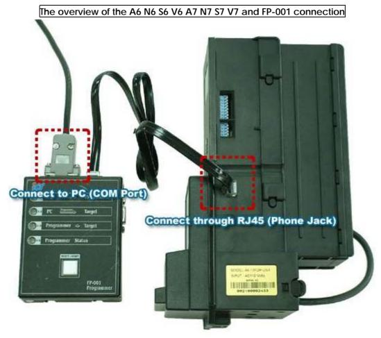
The overview of the U70(px) U77(px) U85 B70UF B77UF B85UF and FP-001 connection
