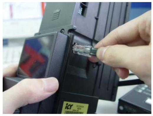
(1.6) Plug the WEL-7U03 another connector to the BA firmly. For model U70(px) U77(px) U85 B70UF B77UF B85UF
