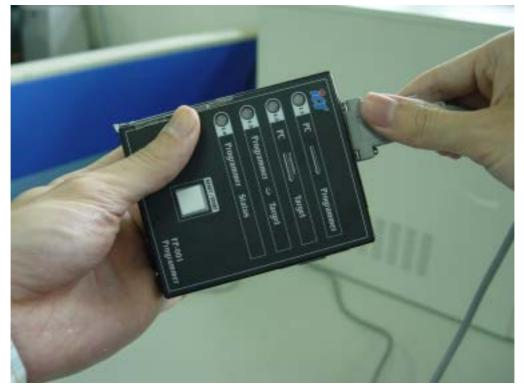
1.5 Plug the harness RJ45 connector to the Download Board FP-001. Harness WEL-M009 is for A6 N6 S6 V6 A7 N7 S7 V7. Harness WEL-7U03 is for U70(px) U77(px) U85 B70UF B77UF B85UF.
