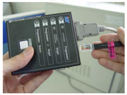
1.6 Plug the WEL-M009 another RJ45 connector to the BA firmly. For model A6 N6 S6 V6 A7 N7 S7 V7.
