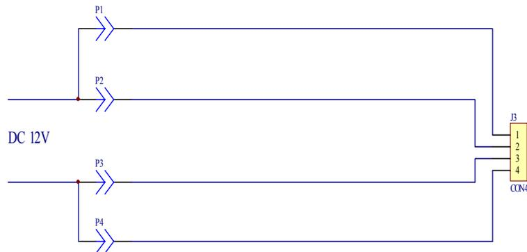
(3) Main power supply & charging capacitor wiring diagram
