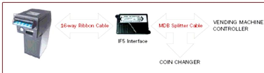
Figure 5 - Connecting the NV200 in MDB mode
