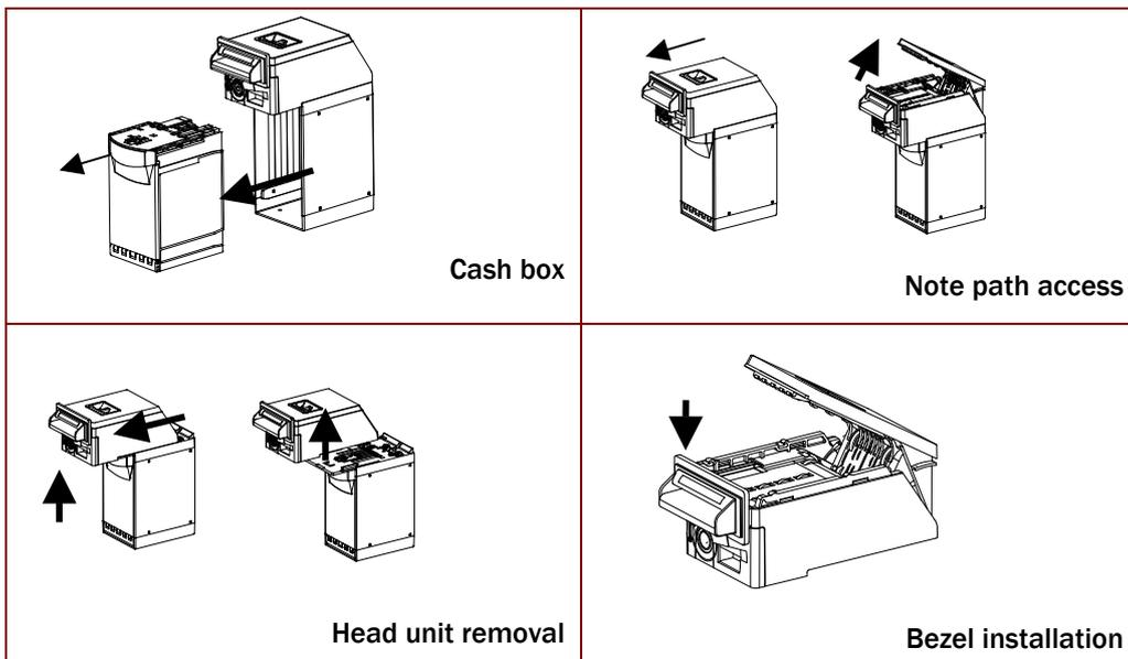
In the Appendix B – NV200 Mechanical Installation you can find a detailed explanation for cash box removal, note path access, bezel installation and validator head unit removal.
