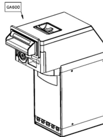
1. OPEN THE LID OF VALIDATOR ASSEMBLY (PA621) BY FIRST SLIDING FORWARD THE HANDLE ON TOP, PLUG IN THE CABLE OF BEZEL ASSEMBLY (PA610) THEN CLICK IT DOWN INTO PLACE, CLOSE LID.
