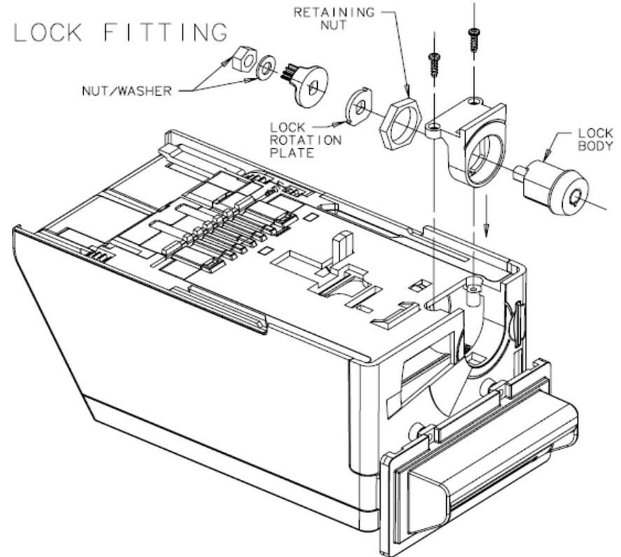
1. UNSCREW 2 OFF SCREWS (INDICATED) WITH A T8 TORX SCREWDRIVER
