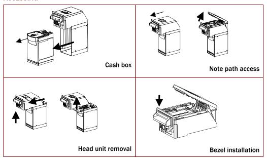
In the Appendix B – NV200 Mechanical Installation you can find a detailed explanation for cash box removal, note path access, bezel installation and validator head unit removal.
