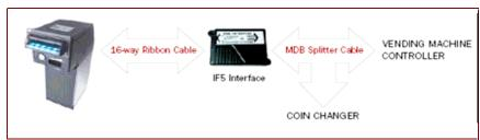
Figure 5 - Connecting the NV200 in MDB mode
