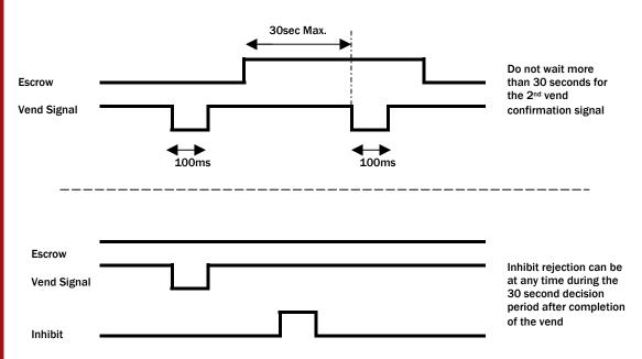
Figure 10 - Escrow Timing Diagram
