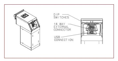
Figure 3 - Connector And Switch Location
