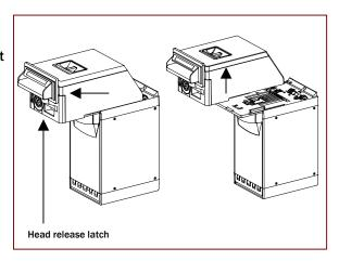
Figure 9 - Validator head removal
