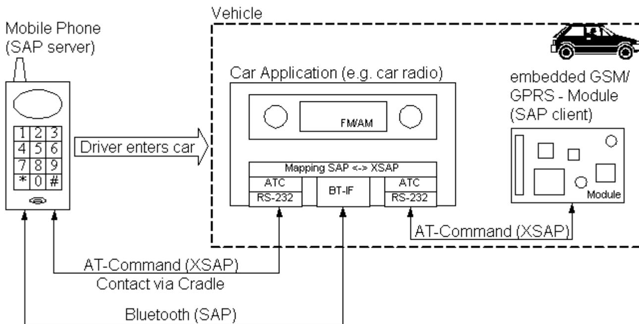
Figure 15.1: Basic Remote SIM Access Usage Scenario
