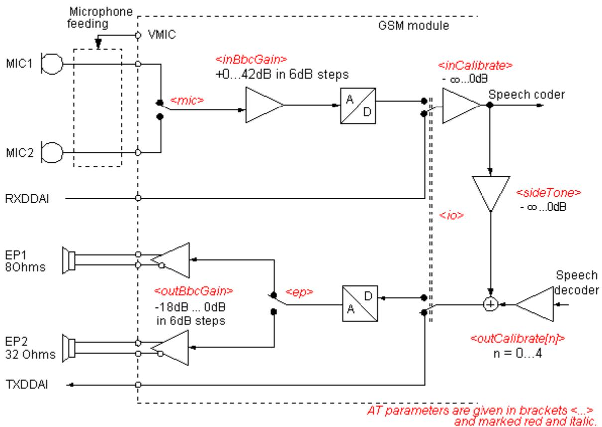
Figure 18.1: Audio programming model for TC65 Module
