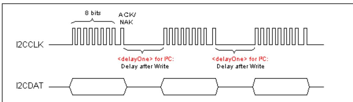
Figure 19.2: Delay time on I<sup>2</sup>C after Write
