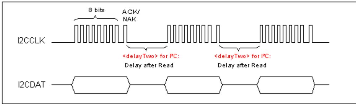
Figure 19.3: Delay time on I<sup>2</sup>C after Read
