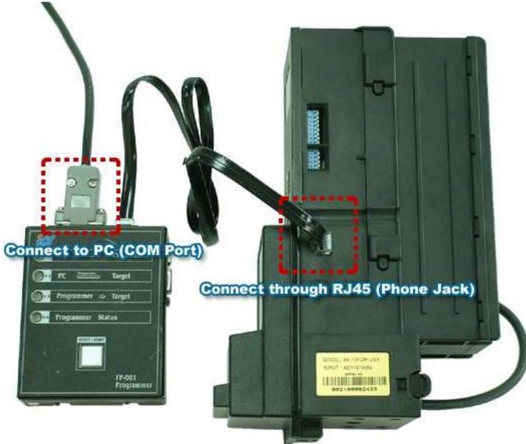
The overview of the U70(px) U77(px) U85 B70UF B77UF B85UF and FP-001 connection
