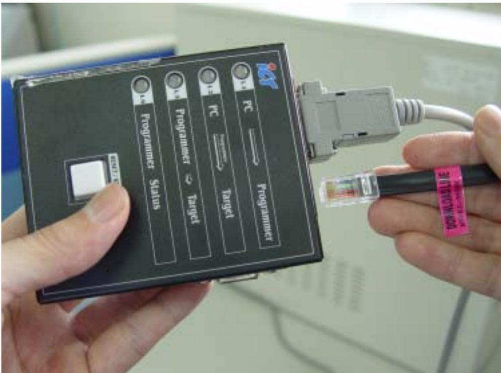
1.6 Plug the WEL-M009 another RJ45 connector to the BA firmly.
