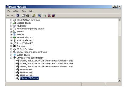
**Figure 15:** Zytronic USB Sensor connected and displayed in the Windows Device Manager
