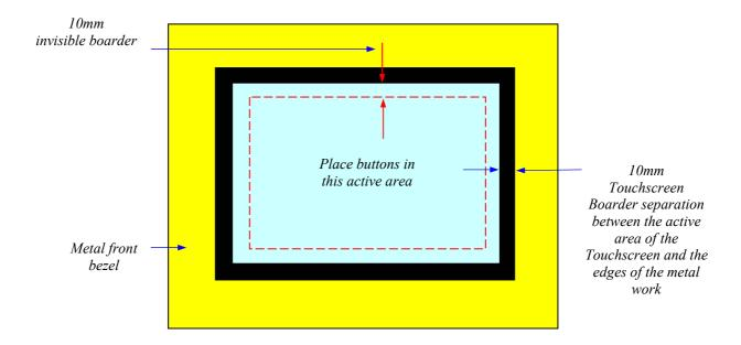
**Figure 4:** Recommended Metal bezel spacing and activation button placements
