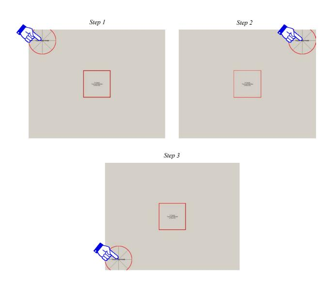
**Figure 24:** Three target calibration screens. Apply and hold a touch on the centre of each of the targets
