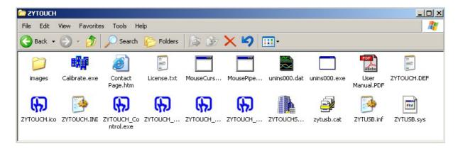
**Figure 40:** ZYTOUCH® Projected Capacitive Driver files with Touchscreen configuration data stored in the ZYTOUCH.ini file
