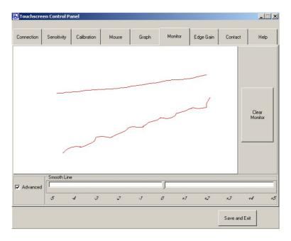
**Figure 33:** *Example of Inter-Wire Linearity adjustment (Line Smoothing)*
