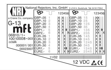
**Example** – Inhibit a currency as coin group X The coin validator must only accept euros and no longer the British currency
