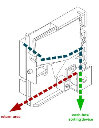
Fig. 2b: Coin acceptance and rejection path of the front entry model
