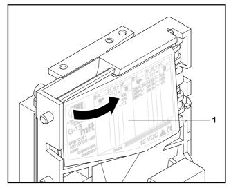
Fig. 7: Open the flight deck of the coin validator.
