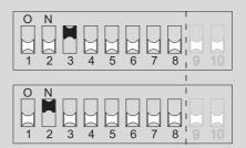
With the DIL switches in these positions, the coin validator no longer accepts the coin type(s) assigned to coin channels 3 and 10!
