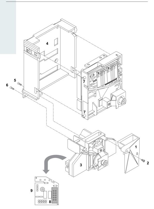
Fig. 4b: Connect G-13.mft, top entry model, to NRI sorting device
