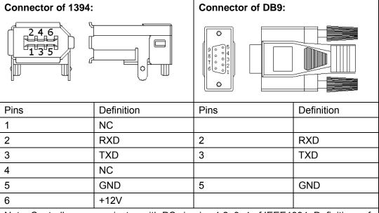
Note: Controller communicates with PC via pins 1,2, 3, 4 of IEEE1394. Definitions of the pins refer to those of PC.
