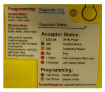
The Diagnostic Button on top of the Geo Gravity is capable of several functions:
