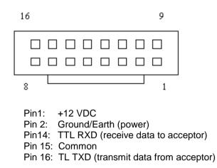
For complete technical detail on the RS232 interface, refer to manual 254053002
