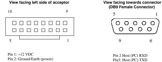
Pin 14: RXD (received data acceptor) Pin 15: Common Signal
