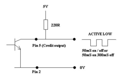
Pulses/Denomination:Factory set per customer specification or via<br/>GFlash program.Pulse Output Rate:High: 50 msec ON/50 msec OFF<br/>Low: 100 msec ON/300 msec OFF
