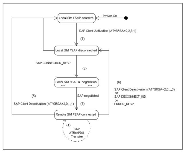
Figure 15.3: SIM usage states of SAP client
