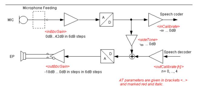
Figure 18.2: Audio programming model for TC65 Terminal
