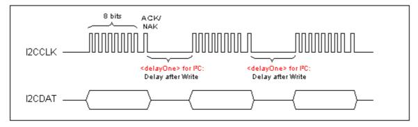
Figure 19.2: Delay time on I<sup>2</sup>C after Write
