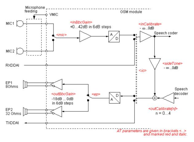
Figure 18.1: Audio programming model for TC65 Module
