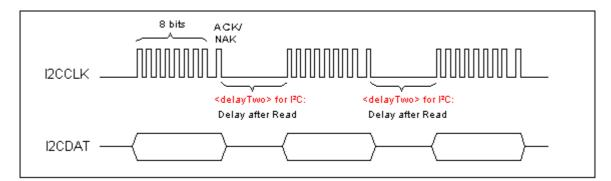
Figure 19.3: Delay time on I<sup>2</sup>C after Read
