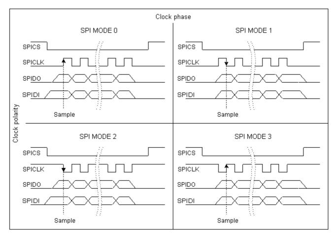
Figure 19.4: SPI modes selectable on SPI
