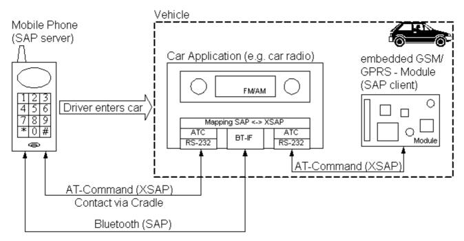
Figure 15.1: Basic Remote SIM Access Usage Scenario
