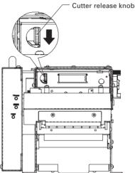
4. When the control box is set apart from the printer, turn the cross hole shown in the figure in the arrow direction to restore the blade.
