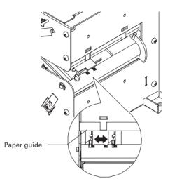
3. When using the paper holder (PHU-3\*\*\*), loosen the screws (4 places including other side) shown in the figure, adjust the holder to the specified width, and then tighten the screws.
